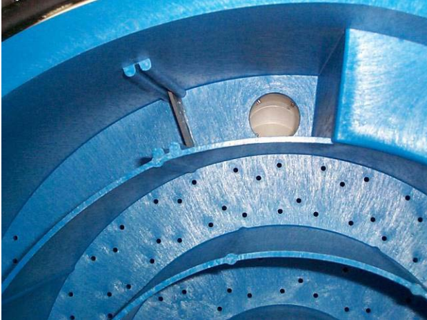
Figure 10 – The Clearadon has large 3/16" holes in the aeration tray that won't scale over with minerals.
