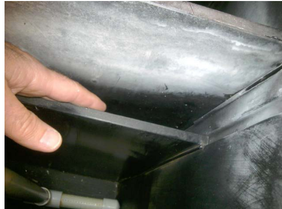
Figure 9 - This is one of two slotted confined areas in the aeration chamber of the AIRraider with no easy way to be clean.
