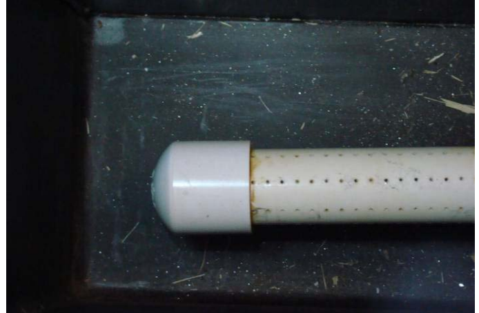
Figure 11 – See the 1/16" holes in AIRRaider system which are prone to being plugged with minerals.
