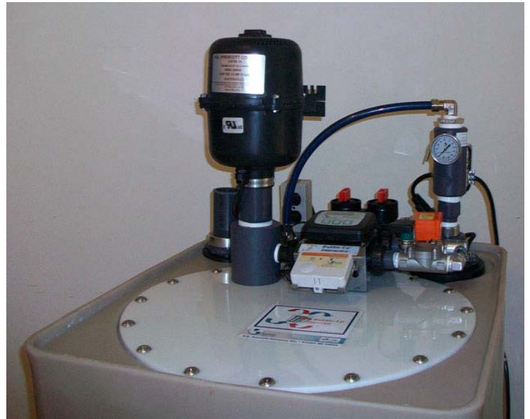
Figure 7 – Let's count the screws and others things to remove for access for cleaning the Bubble-Up.
